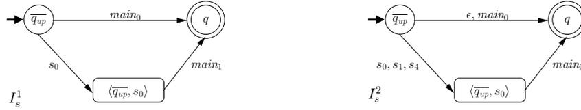
Fig. 1.12. Automata representing the set  $I_s^1$  and  $I_s^2$  of skyline configurations reachable within one, respectively two, steps from the initial configuration.
