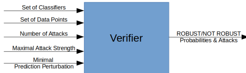
Fig. 1. The verifier takes as input a set of classifiers, a set of labelled data points, the number of attacks, and the attack properties. If the verifier does not find a solution, we can be sure is robust against any attack with the specific properties. Otherwise, it returns the optimal attack.
